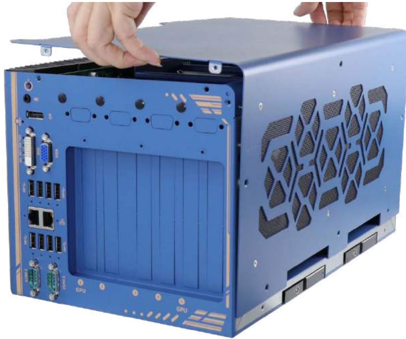
Place L-shape side panel onto the enclosure
