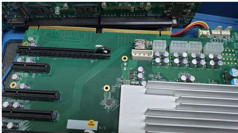
Disengage the daughter-board from the motherboard
