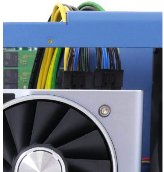
6 or 8/ 8-pin power connector on graphics card
